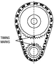
Figure 1— Timing Chain Sprocket Alignment
